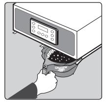
5 Slide the filled brew basket into the brew rails under the control panel. Slide it all the way back until it stops.
