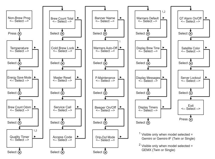
**Temperature -** sets the brewing temperature of the water held in the water tank. The factory default setting is 200°F/92°C (Gourmet STD). The setting range is 170°F to 206°F (77°C to 97°C). Once accessed, press ◀ or ► to choose the desired temperature. Then press o to set and exit.
