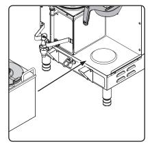
2 Place an empty satellite under the brew basket. Make sure the satellite is pushed all the way back against the front cover.
