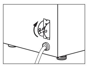
12 Once the water tank is full (you will hear the water stop flowing), turn off the power switch and disconnect the power cord.
