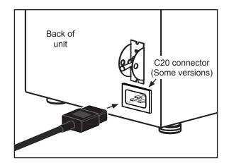
9 Make sure that the power switch is off, then connect the power plug to the appropriate type of electrical outlet.
