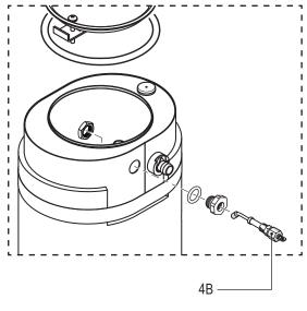
Water Level Probe Detail (Older Units)
